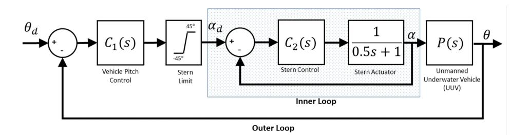
In this example an inner-loop controller is used to control the pitch of the stern plane. An outer-loop PD controller is used to control the pitch of the vehicle and feeds into the inner loop.
