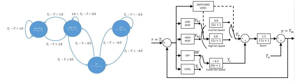
In this example we take the heating and cooling example a little further by introducing a more complex system where the system has a heater, cooler, and variable speed fan. The different elements of the system require different control strategies and even actuators, and thus hybrid control is a perfect fit.
